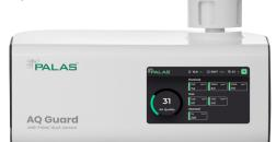
AQ Guard, currently the most advanced compact analyzer for determining indoor air quality, continuously and reliably analyses airborne fine dust particles in the range 0.175 – 20  $\mu$ m (<sup>\*1</sup> IAHP-Package starting from 0.15  $\mu$ m). A newly developed mass conversion algorithm calculates PM values based on single particle optical light scattering, considering signal duration and shape.
